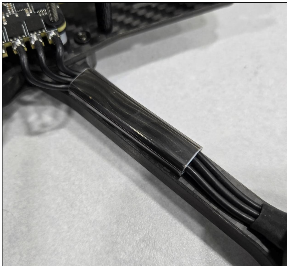
Figure 16: Cable Management Placement
