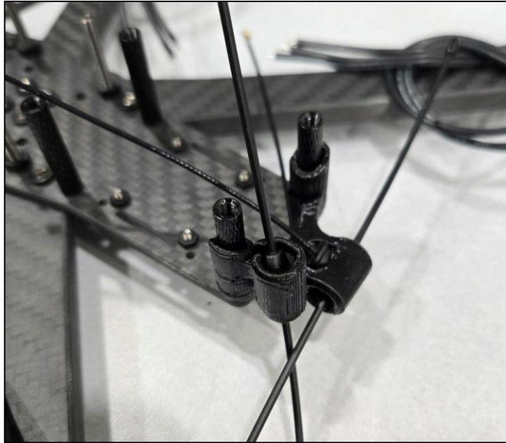
Figure 9: Antenna Mount Placement
