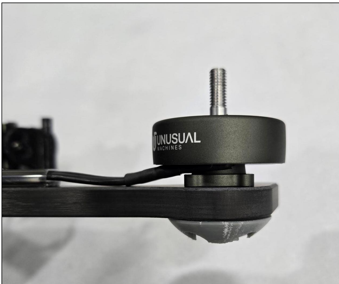
Figure 4: Motor and Motor Cap Installation
